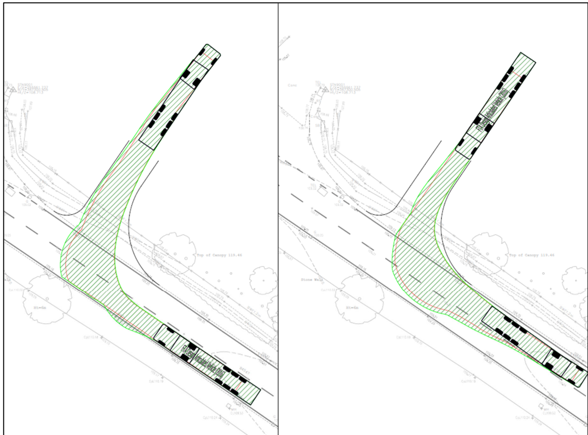
Figure 2.3 Swept Path Analysis of Site Access
