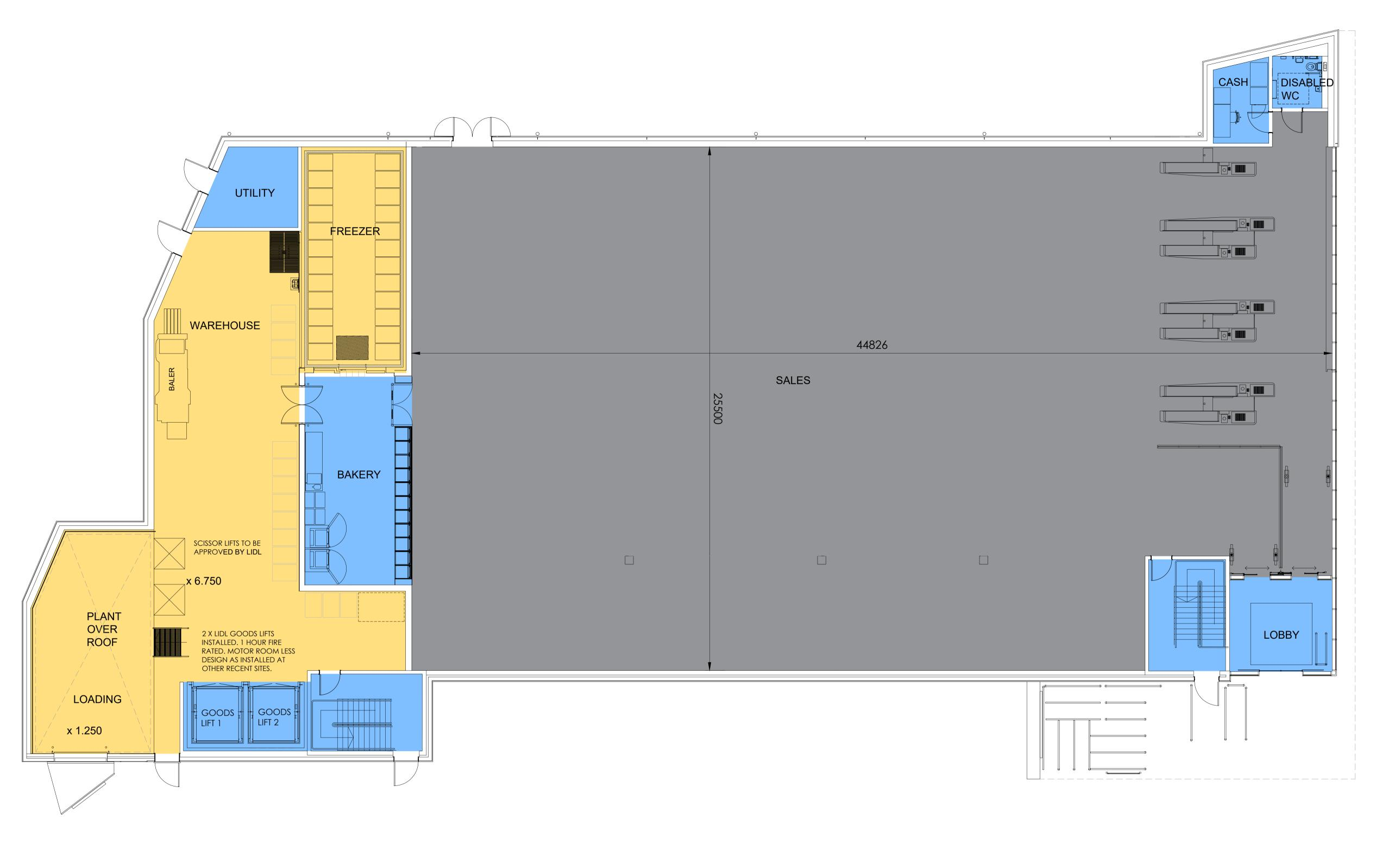
SCHEDULE 1102 m<sup>2</sup> Sales Area GF Warehouse 295 m<sup>2</sup> 170 m<sup>2</sup> GF Ancillary 19 m² Internal Wall 1586 m<sup>2</sup> GF GIA GF GEA 1675 m² 119 m² FF Ancillary 315 m<sup>2</sup> FF Warehouse 9 m<sup>2</sup> Internal Wall FF GIA 443 m² FF GEA 519 m² 2029 m² Total GIA Total GEA 2194 m<sup>2</sup>
